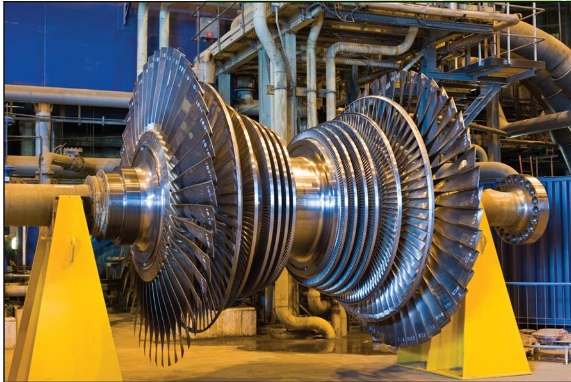
Figure 1.9: Rotor assembly of a turbine showing multiple stages of turbine blades.
